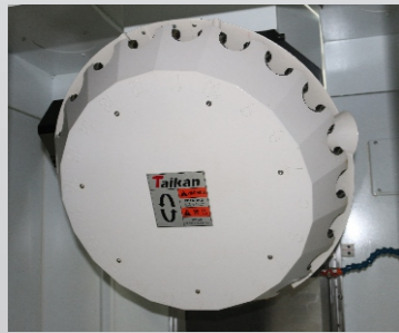
21T- Adopt Mitsubishi servo motor, equipped with M80A system ,to improve response speed and stability of tool magazine .Tool changing is only 1S.
