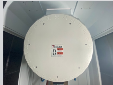
26T-Tool to Tool 1.35S,large capacity of tool magazine to satisfy a machine to complete all processes,and support Max 3Kg.
